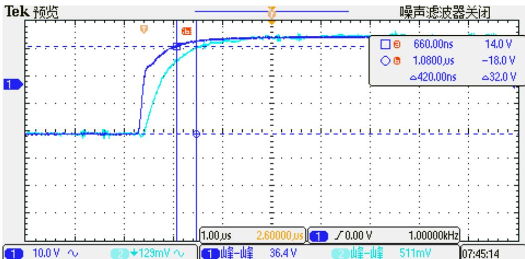
Figure 5. The typical frequency response of STK-616AMF2 series current sensor. The response time from 90% of the primary current to 90% of the secondary output is 0.5  $\mu$ s.
