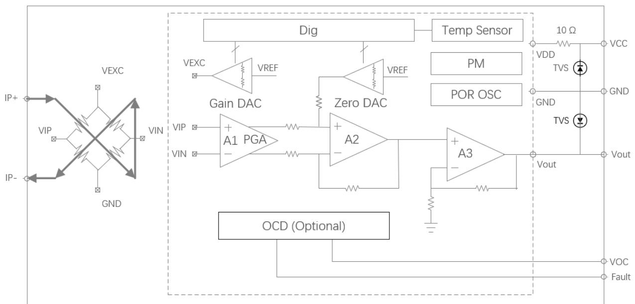
Figure 6. The functional block diagram for the STK-616AMF2 series products.
