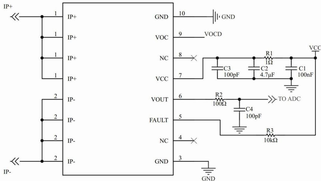
Figure 7. The reference application circuit for the STK-616AMF2 series products.
