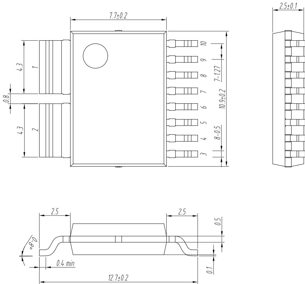
Figure 2. Dimensions of STK-616AMF2 series current sensors. The unit is mm.
