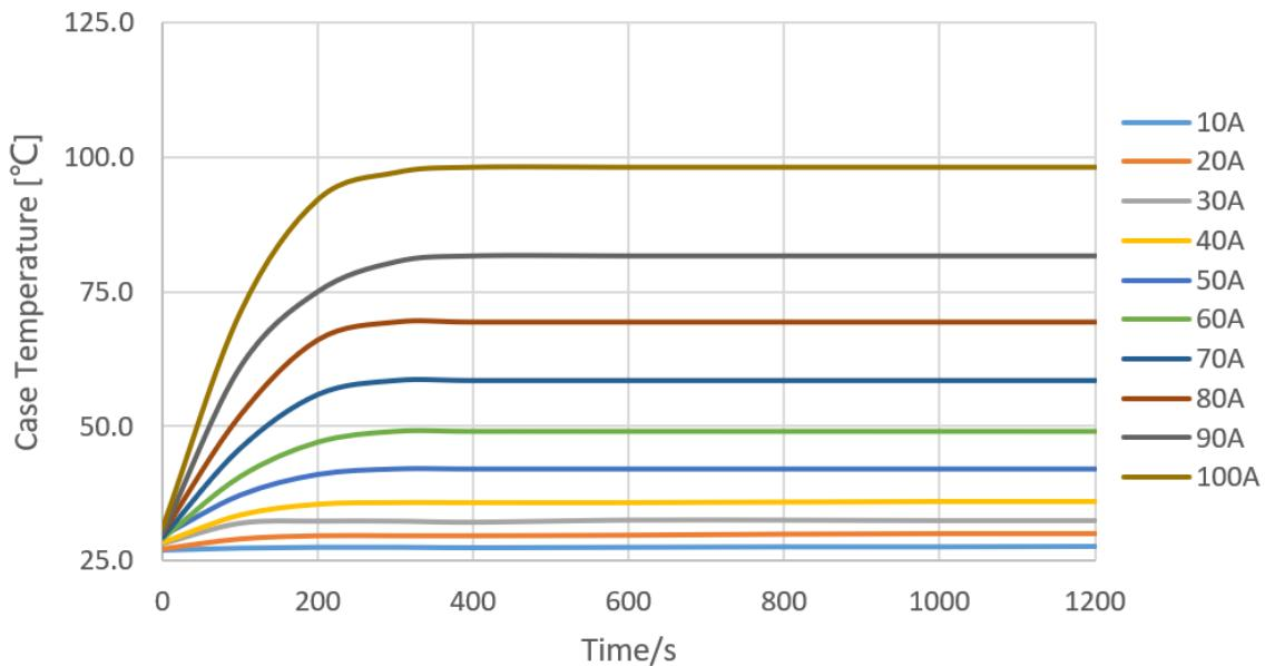
Figure 1. Relationship between STK-616AMF2 Case temperature and amount of input current.
