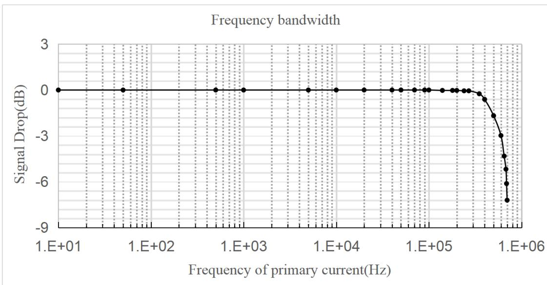
Figure 4 the frequency band width of the STK-616AMF2 series products. the upper limit of the -3 dB band width is 500 kHz.
