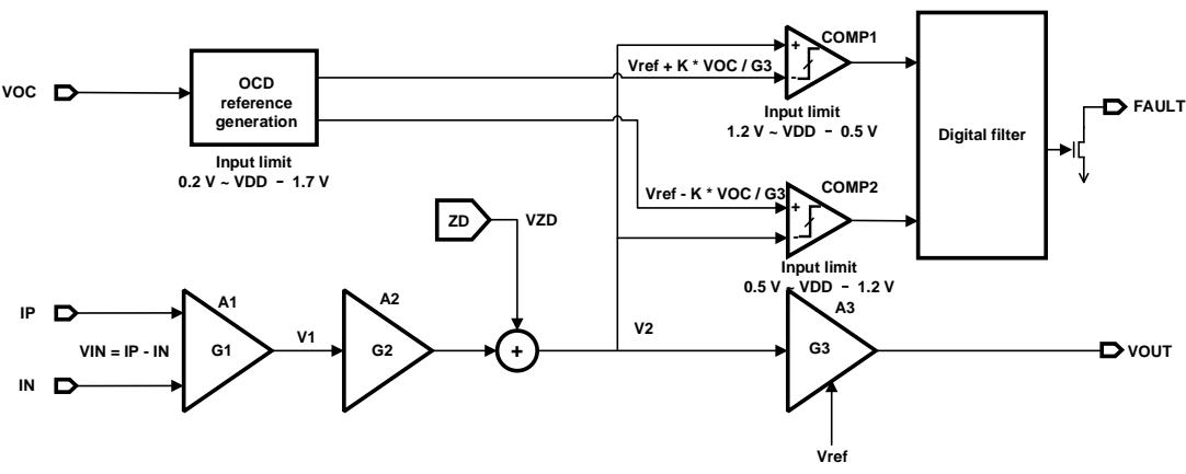
Figure 11 the functional block diagram for STK-616AMF2 on OCD function with conditions of  $V_{cc} = 5 \text{ V}$ ,  $V_{off} = 2.5 \text{ V}$ ,  $V_{ref} = 2.5 \text{ V}$ .
